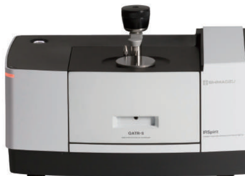
Fig. 3 QATR-S Accessory Installed in IRSpirit Sample Compartment
