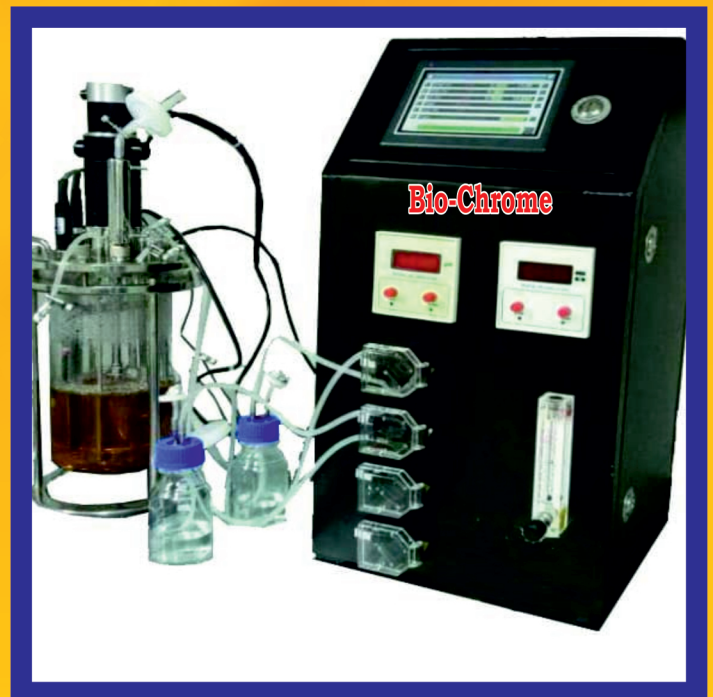
PLC TOUCH SCREEN BASED FERMENTER
